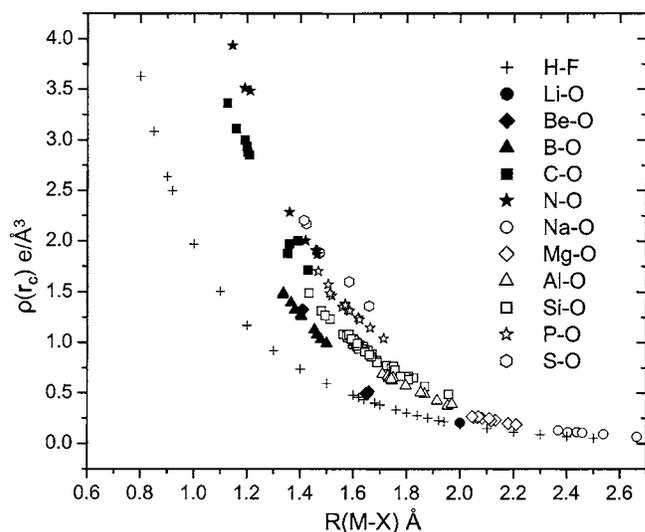
FIG. 1. Scatter diagrams (a) of the value of the electron density,  $\rho(\mathbf{r}_c) \times (e/\text{\AA}^3)$ , evaluated at the  $(3,-1)$  bond critical points  $\mathbf{r}_c$  vs the bond lengths,  $R(M-X)$ ( $\text{\AA}$ ), for  $M$ -O bonded interactions (Ref. 14) involving first- and second-row  $M$  atoms bonded to O and H-F bonds for the HF dimer (Ref. 15).
