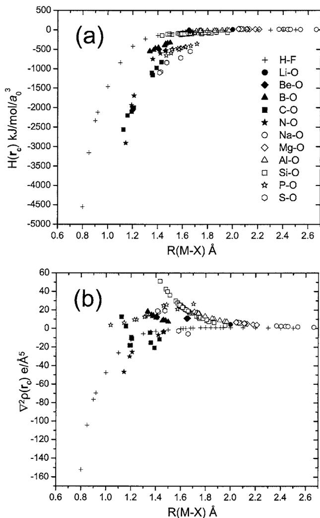
FIG. 3. (a)  $H(\mathbf{r}_c)=G(\mathbf{r}_c)+V(\mathbf{r}_c)$ , the local electronic density energy ( $\text{kJ/mol}/a_0^3$ ) evaluated at  $\mathbf{r}_c$  vs  $R(M-X)$ ( $\text{\AA}$ ) and (b)  $\nabla^2\rho(\mathbf{r}_c)$ , the Laplacian of  $\rho(\mathbf{r}_c)$ ( $e/\text{\AA}^5$ ) evaluated at  $\mathbf{r}_c$  vs  $R(M-X)$ ( $\text{\AA}$ ).
